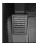
The parking brake pedal is located to the left of the regular brake pedal, near the driver's door.
